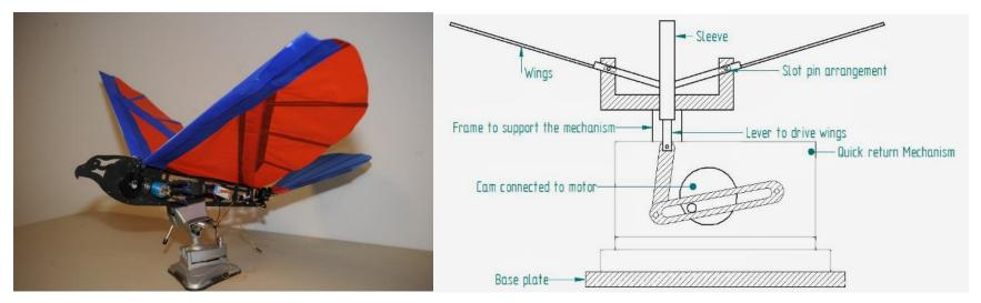
An ornithopter is a type of aircraft that flies by flapping its wings, mimicking the flight of birds and insects. Unlike airplanes, which generate lift through the forward motion of fixed wings or rotors, ornithopters generate lift and propulsion by flapping their wings in a motion similar to birds.
