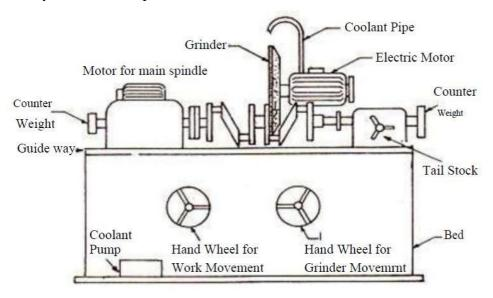
The grinding wheel is driven by a separate motor. A coolant pump is provided with a flexible pipe line to supply the coolant at the cutting zone. Counter weights are provided at head stock and tail stock to balance the crank shaft.
