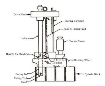
Before starting reboring operation it is very important to prevent the entry of metal or abrasive particles in the oil galleries. It is a good practice to warp insulation tapes on crank pins and to cover other parts as is possible.
