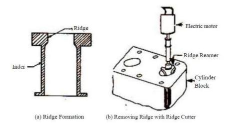
This ridge if found must be removed before proceeding further, because otherwise the rings are liable to break once the attempt is made to take out the piston rod assembly from the top. The ridge is removed by means of a special ridge reamer.
