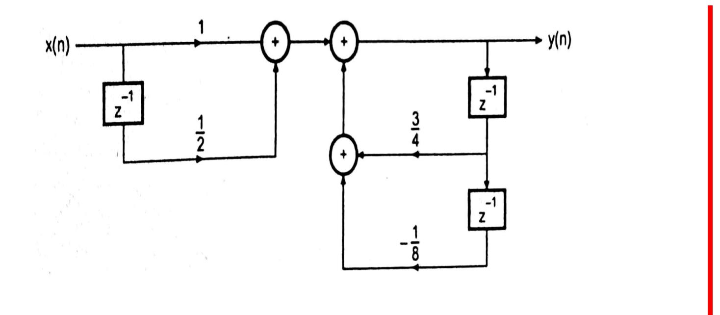
REALIZATION STRUCTURES FOR IIR FILTERS 19ECB212 – DIGITAL SIGNAL PROCESSING/J.PRABAKARAN/ECE/SNSCT
