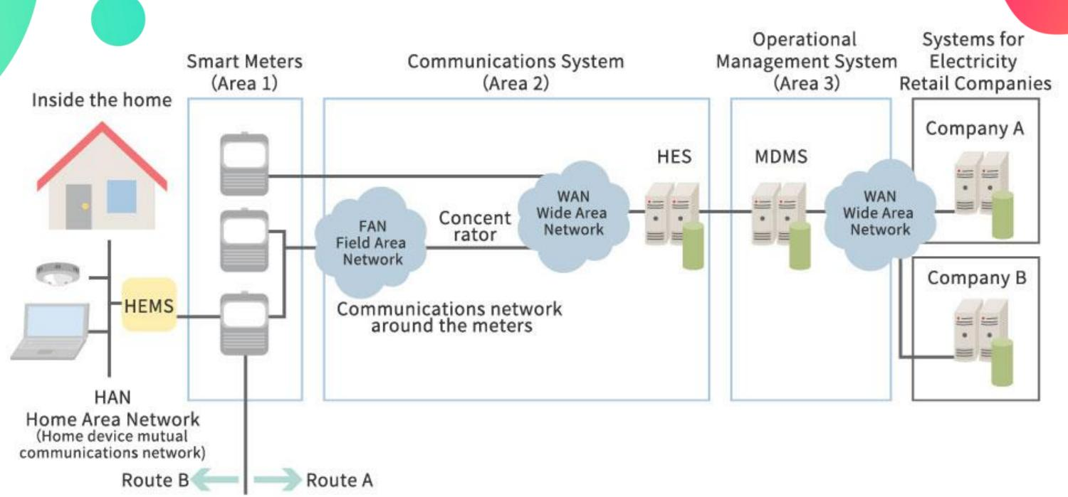
HES: Head-End System (a device that collects data and controls communication)
