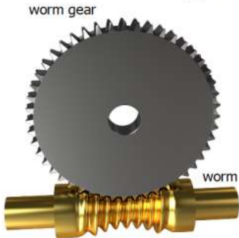
screw gears (hyperboloid gears)
