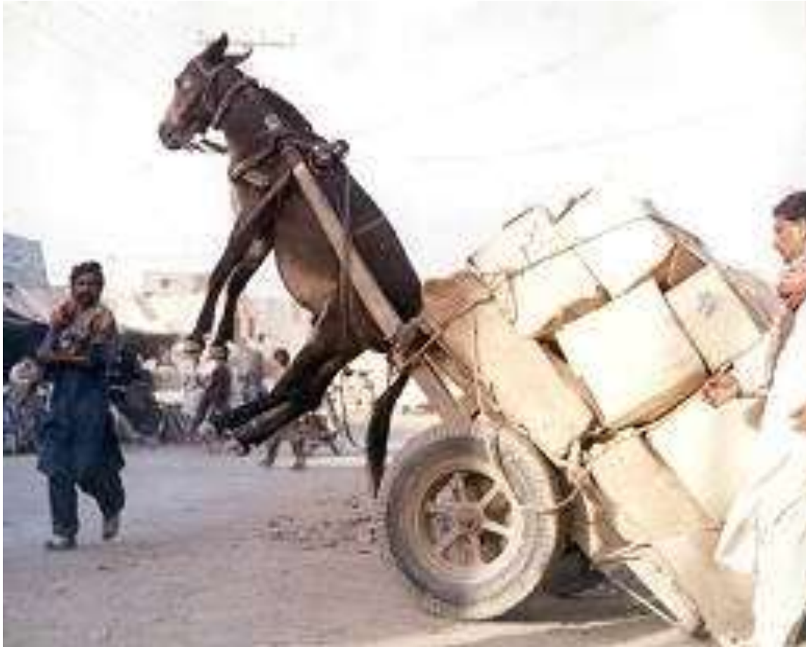
An extreme example of poor load distribution
