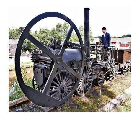
A flywheel acts as an energy reservoir, which stores energy during the period when the supply of energy is more than the requirement and releases energy during the period when the requirement is more than the supply.
