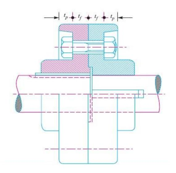
the protruding bolts and nuts are protected by flanges on the two halves of the coupling, in order to avoid danger to the workman
