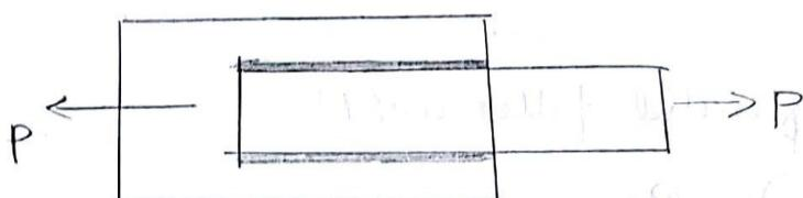
Load & Weld directions are parallel to each other is called Double Parallel Fillet Weld.
