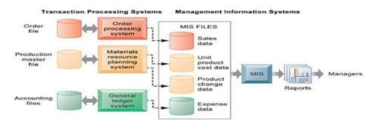
In the system illustrated by this diagram, three TPS supply summarized transaction data to the MIS reporting system at the end of the time period. Managers gain access to the organizational data through the MIS, which provides them with the appropriate reports.
