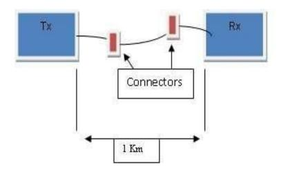
System Power budget (Min. received Signal level)= 14 dB Actual received power( due to Link loss ) = 2.5 dB Link Margin = 12.5 dB
