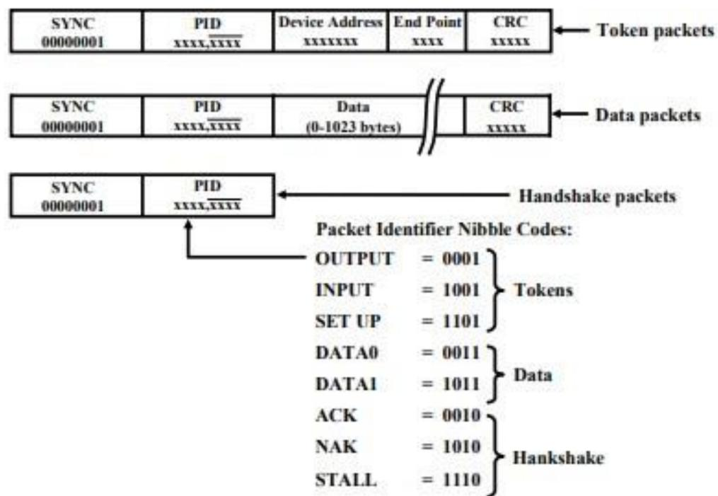
Fig. 5 Examples of the various kinds of USB signaling and data packets.
