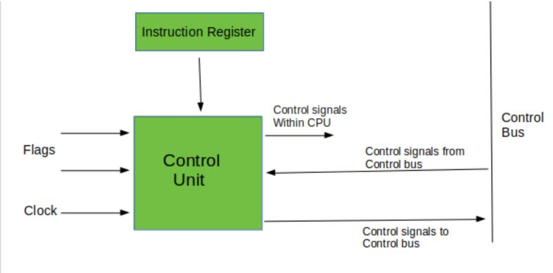
Block Diagram of the Control Unit
