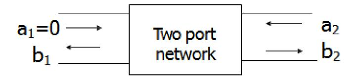
$$S_{22} = \frac{b_2}{a_2} = \text{reflection coefficient at port 2 with a }_{1} = 0$$
