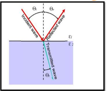
➤ Reflection is the result of digital TV signal hitting on obstructions with properties (thickness, length) much larger than the wavelength of the radio wave (e.g. smooth surface of walls and hills/mountains)
