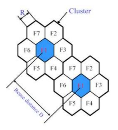
For hexagonal cells, the reuse distance is given by
