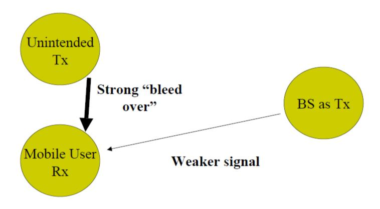
The Mobile receiver is captured by the unintended, unknown transmitter, instead of the desired base station
