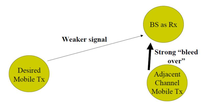
The Base Station faces difficulty in recognizing the actual mobile user, when the adjacent channel bleed over is too high.
