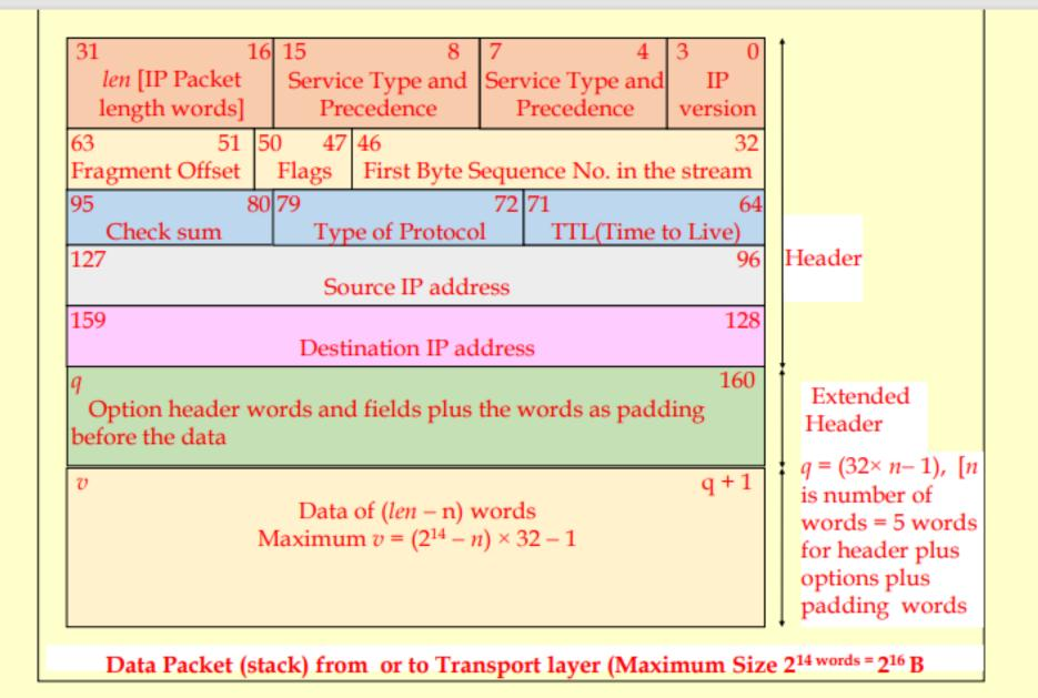
Fig. 4.3 Data stack received or transmitted at or to transport layer and packet consisting of IP header fields of 160 bits and extended header (n - 5) words (when required) plus data stack of maximum v words from or for the transport layer
