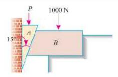
If the angle of friction for all the surfaces is 14°, find graphically the force (P), which should be applied to the wedge. Also check the answer analytically.
