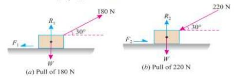
Now consider a push of 220 N acting on the body. We know that in this case, the force of friction  $(F_2)$  will act towards right as shown in Fig. 8.3 (b).
