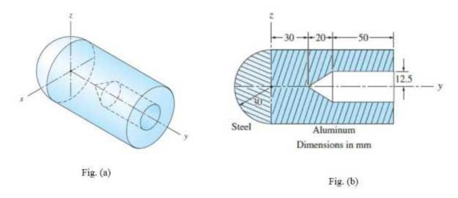
By symmetry, we note that  $\bar{x} = \bar{z} = 0$ . If the machine part were homogeneous, its center of mass would coincide with the centroid of the enclosing volume, and  $\bar{y}$  could be determined using the method of composite volumes.
