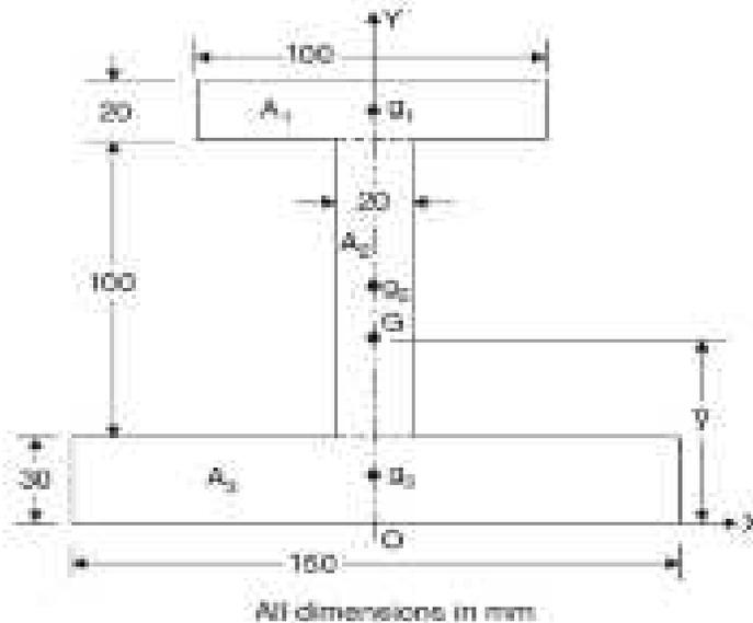
*Solution:* Selecting the coordinate system as shown in Fig. ... due to symmetry centroid must lie on y axis,
