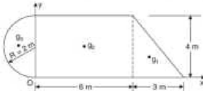
**Solution:** The composite section is divided into three simple figures, a triangle, a rectangle and a semicircle
