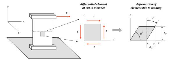
Shear strain deformations produce skewing in a rectangular-shaped stress element: the angle between adjacent sides changes from  $\pi/2$  to  $\theta^*$ . Here, we will define the shear strain as  $\gamma$  representing this change in angle:
