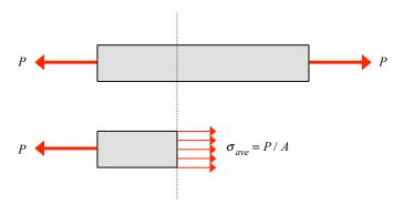
Since the axial load throughout the rod is P, we can write down that the average axial stress is the axial force divided by the cross-sectional area:
