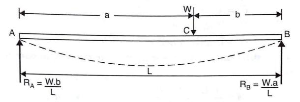
The above equation of B.M. holds good for the values of x between 0 and 'a'. The bending moment at any section between C and B at a distance x from A is given by,
