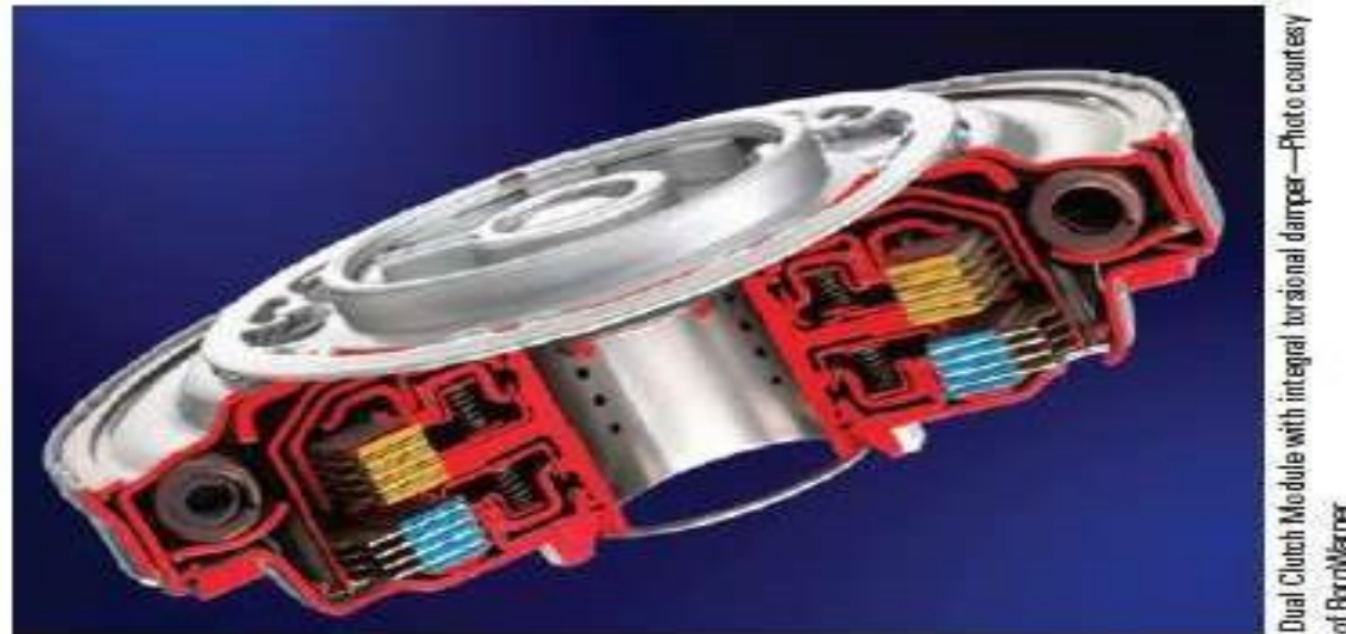
Figure 69.23 A dual clutch transmission employs two clutches that alternately connect engine output to transmission input shafts for odd-numbered gears or even-numbered gears, respectively.
