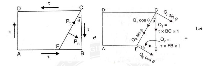
Angle made by oblique section FC with normal cross section BC,
