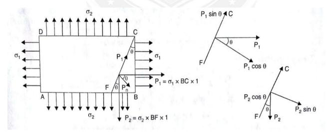
Fig. shows a rectangular bar ABCD of uniform cross sectional area A and of uniform thickness. The bar is subjected to two direct tensile stresses (or two principal tensile stresses) as shown in Fig
