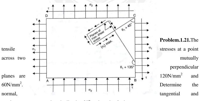
resultant stresses on a plane inclined at  $30^{\circ}$  to the axis of minor stress
