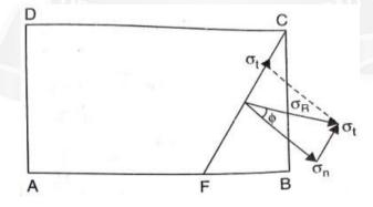
**Maximum Shear stress**. The shear stress is given by  $\sigma_t = \frac{(\sigma_1 - \sigma_2)}{2} \sin 2\theta$ . The shear stress
