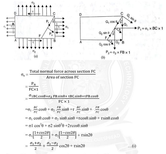
Tangential stress (i.e., shear stress) across the section FC,
