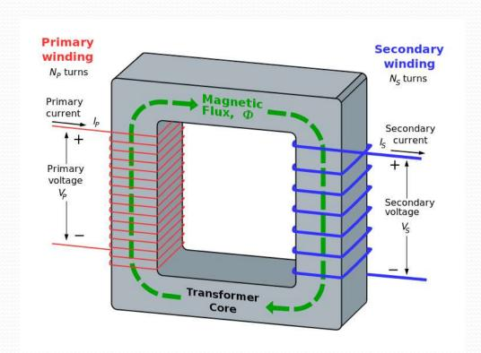
The primary winding is connected to the single – phase ac supply, an ac current starts flowing through it
