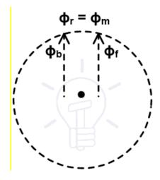
Now consider after the rotation of  $90^{\circ}$ , both filed are rotated and pointing in the same direction. Therefore, the resultant flux is a summation of both fields.
