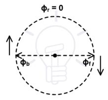
When a motor starts, two fields are induced as shown in the above figure. These two fields are the same magnitude and opposite direction. So, resultant flux is zero.
