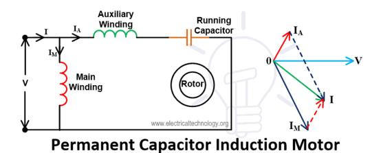
The power factor and efficiency of this motor are very high and also it has a high starting torque that is 80% of full load torque.
