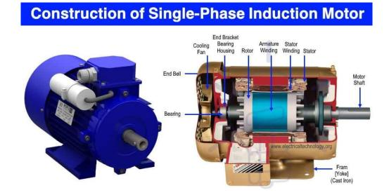
Similar to a three-phase induction motor, single-phase induction motor also has two main parts;
