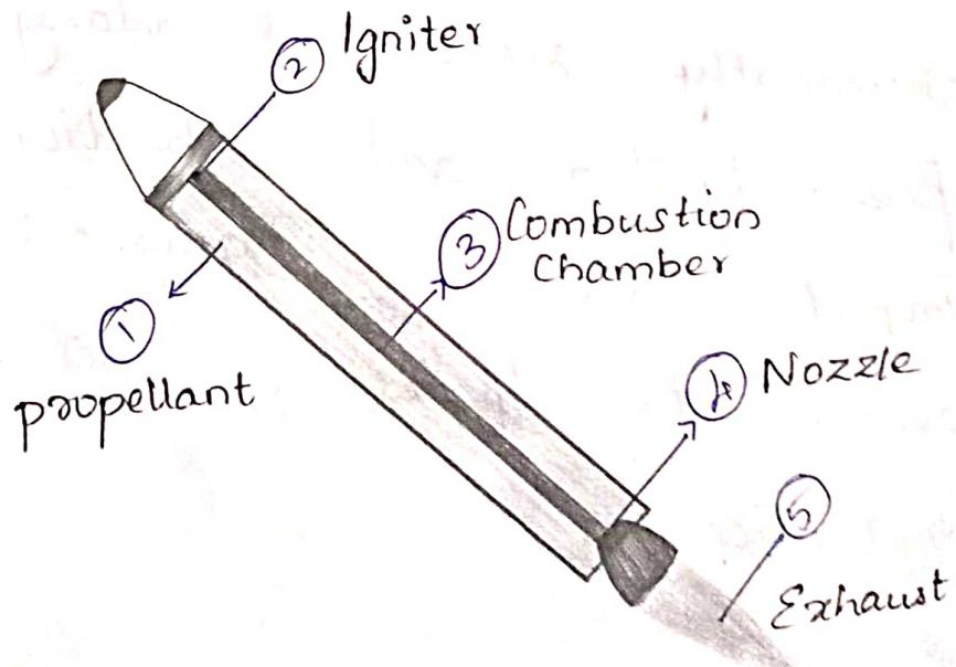
① → A solid fuel-oxidizer mixture (propellant) is packed into the rocket, with a cylindrical hole in the middle.
