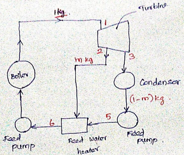
The steam expands from condition 1 through the turbine. At the pressure corresponding to point 2, a quantity of steam with  $m$  kg per kg of steam supplied from boiler is bled off for heating feed water. The rest of steam  $(1-m)$  kg completes the expansion and is exhausted to the condenser pressure  $P_3$ . The amount of steam is then condensed and pumped to the same pressure as the bleed steam. The bleed steam of  $m$  kg and feed water are mixed in the feed water under
