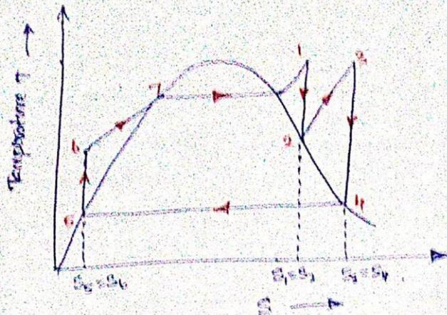
The process 1-2 represent isentropic expansion in high-pressure turbine, and 3-4 represent isentropic expansion in low-pressure turbine. The steam is reheated at constant pressure 2-3. The reheat can be carried out by returning the steam to the boiler and passing it through a heat exchanger placed in the boiler at constant pressure.
