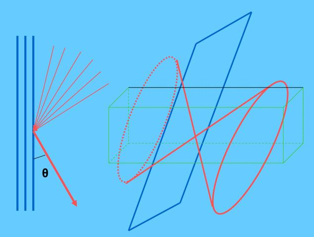
Inelastic scattering without significant wavelength change leads to formation of Kikuchi lines by diffraction. Incoming beam has every possible direction. Outgoing strong beam is at Bragg angle. This is particularly seen in thick samples
