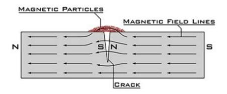
But when a crack or other discontinuity is present, the magnetic flux leaks out of the material. As it leaks, magnetic flux (magnetic field) will collect ferromagnetic particles (iron powder), making the size and shape of the discontinuity easily visible.
