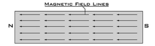
When ferromagnetic material (typically iron or steel) is defect-free, it will transfer lines of magnetic flux (field) through the material without any interruption.
