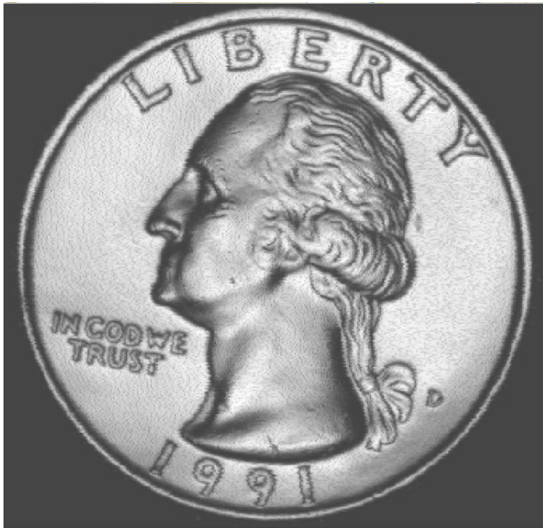
Gray scale image produced using the sound reflected from the front surface of the coin
