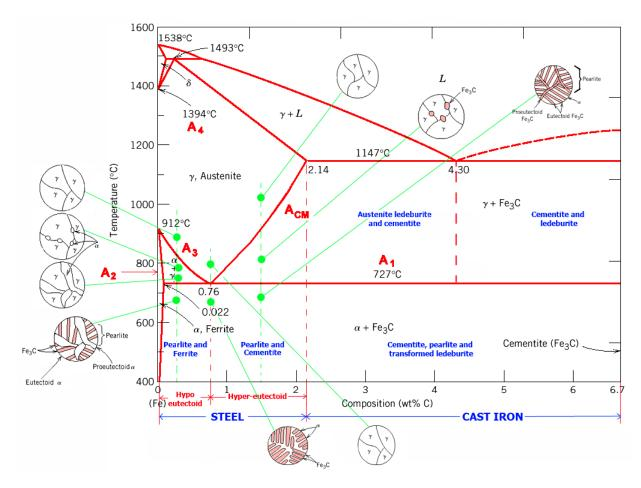
The iron-carbon (Fe-C) phase diagram is a graphical representation of the phases that exist in equilibrium at different temperatures and carbon concentrations in an iron-carbon alloy. This diagram is crucial for understanding the behavior of steels, which are alloys of iron and carbon. The phases in the diagram include ferrite, austenite, cementite, and various phases that form during phase transformations.
