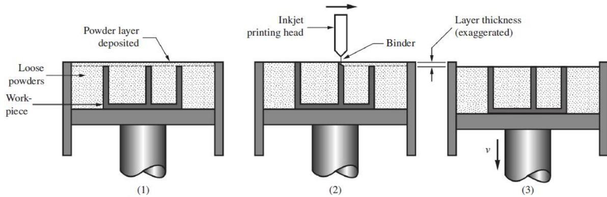
**Figure** Three-dimensional printing: (1) Powder layer is deposited, (2) inkjet printing of areas that will become the part, and (3) piston is lowered for next layer (key: v = motion).
