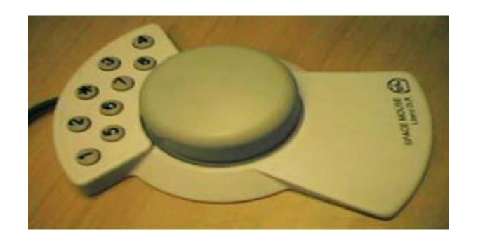
A 3D mouse has two parts as vertical & horizontal part. Each part has some buttons. With different combinations of these buttons the user can produce different positions in the 3D environment.
