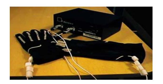
Pinch glove enables natural interaction with objects. It uses hand-signs to execute actions. It continuously tracks the motion of the user's hand & limb and accordingly gives signal to the transmitter.
