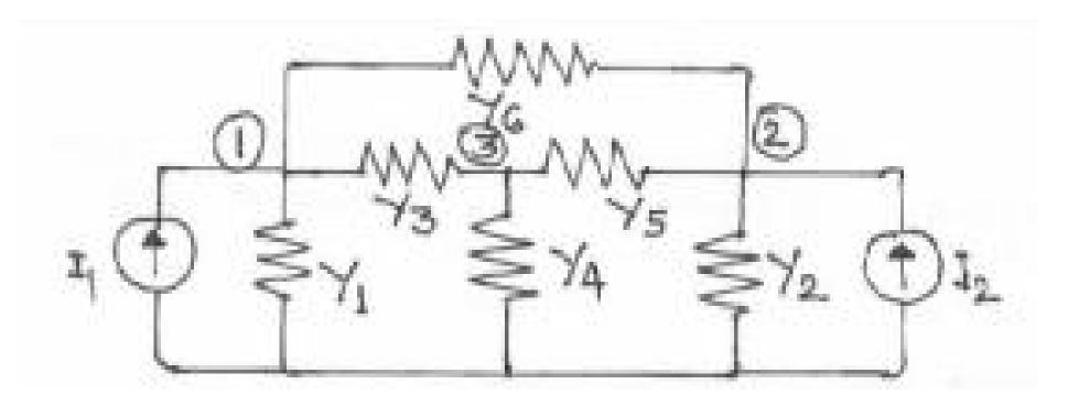
At node 1: I1 = Y1V1 + Y3(V1-V3) + Y6(V1 - V2)
