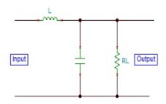
In inductor filter, the ripple factor is directly proportional to the load resistance. On the other hand in a capacitor filter, it is varying inversely with the load resistance. Hence if we combine the inductor filter with the capacitor the ripple factor will become almost independent of the load filter. It is also known as inductor input filter, choke input filter input or LC-section.
