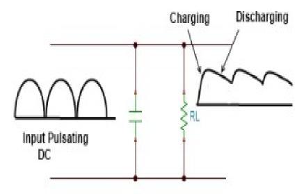
In this filter a capacitor is connected across the load during the rise of voltage cycle it gets charge and this characteristics connected across the load during the fall in the voltage cycle. This process is repeated for each cycle and thus the representation reduced across the load. It is shown in the above Figure. It is popular, because of its low cost, small size, I and good characteristics. Useful for load up to 50mA as in transistor radio battery eliminators.
