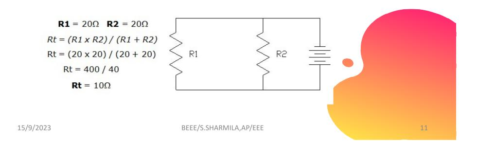
Parallel Circuit Calculations (All Resistors Are the Same)
