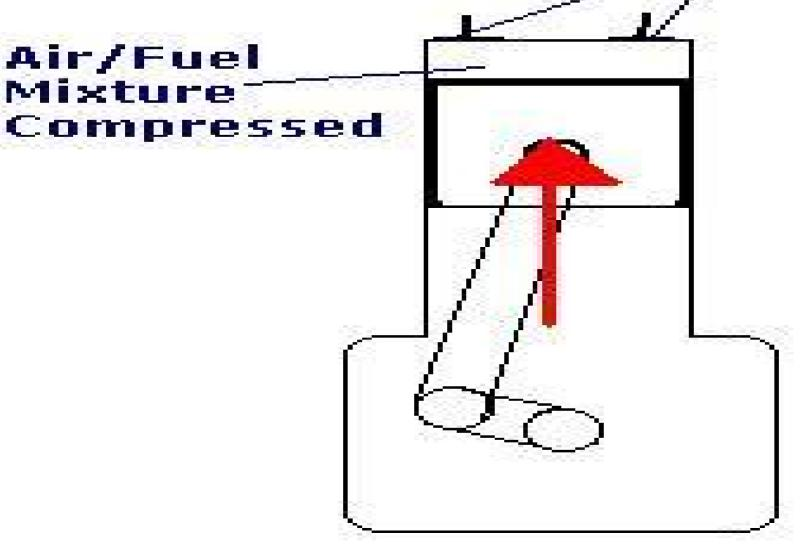
Figure5: Compression Stroke
