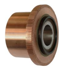
Commutator:--Hard drawn copper bars segments insulated from ea other by mica segments (insulation) -- Between armature & External circuit -- Split-Rings (acts like Rectifier AC to DC)
