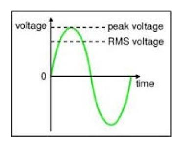
Parameters V and I are in sine wave.
