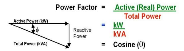
Power Factor is a measure of efficiency (Output/Input)
