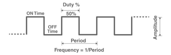
The frequency of PWM determines how fast a PWM completes a period. The frequency of a pulse is shown in the figure above.
