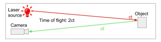
The 3D scanners developed using time-of-flight (TOF) technology captures detailed information about a three-dimensional object using a range imaging camera system. The range imaging camera system resolves the distance between the camera and the real-world object using TOF technology. TOF technology makes the scanner measure the amount of time the infrared light or laser beam takes to reflect back.
