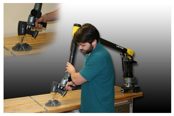
Arm based 3D Scanner and probing system
