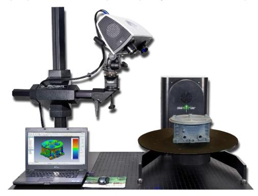
Steinbichler Comet Structured light Blue LED 3D Scanner
