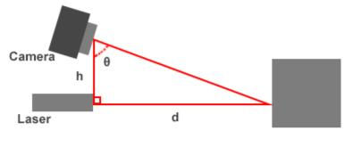
h = distance between camera and laser (known) θ = angle betwen laser and scanner (known) d = distance between scanner and object (unknown)
