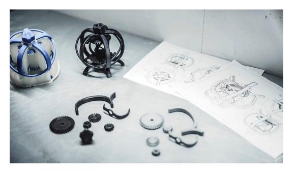
3D printers, like the Zortrax Inventure, can 3D print movable mechanisms as one part accelerating functional testing
