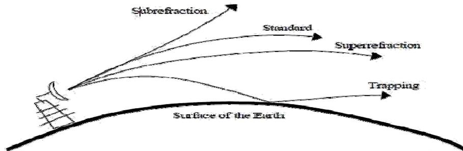
Known as the effective earth radius and it is approximately equal to four-thirds the true radius of the earth (i.e. roughly 8500km). A more classical form of representing  $n$  is that of modified refractivity,  $M$ . In this case, the surface of the earth is represented by a flat plane and the radio rays are constituted by curves that are determined by Snell's law and the corresponding value of  $M$  at each point along the radio link. The following is the expression for  $M$
