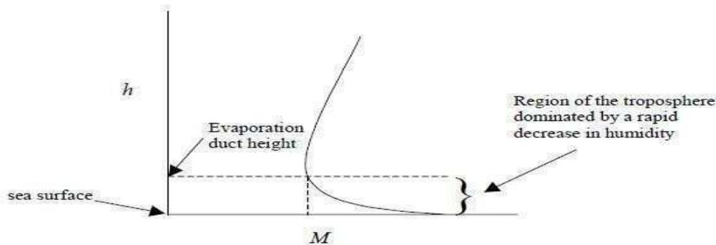
As that portion of the curve with a strong negative  $M$  gradient. Therefore, despite the fact that the height  $h$  is increasing, it is the sharp fall in the water vapour pressure,  $e$ , that contributes to the rapid decrease in  $M$ .
