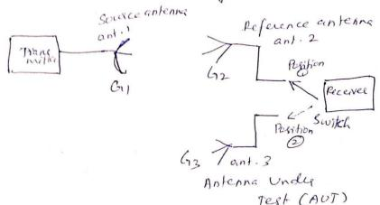
when Switch is at position O, from Friss transmission fermula, [antenna 1 - Tx] antenna 2 - Rx]
