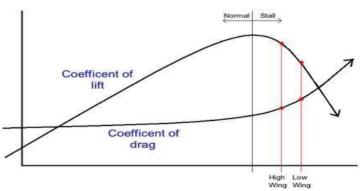
A typical graph of lift coefficient and drag coefficient versus angle of attack. At any angle of attack greater than the stalling angle an increase in angle of attack causes a reduction in lift coefficient and a decrease in angle of attack causes an increase in lift coefficient.
