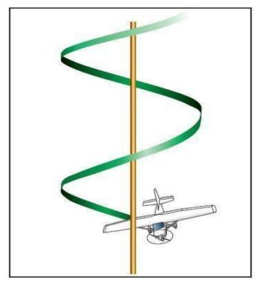
For fixed-wing aircraft, **autorotation** is the tendency of an aircraft in or near a stall to roll spontaneously to the right or left, leading to a spin (a state of continuous autorotation).
